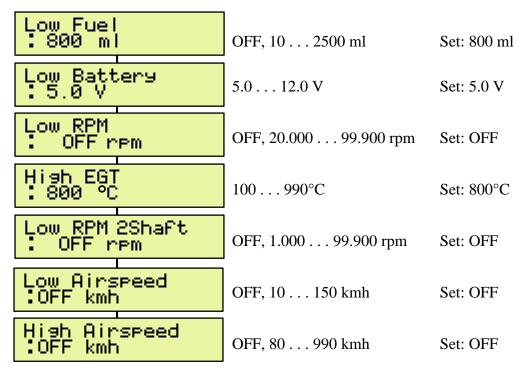
The parameters are largely self-explanatory, lower values as "Low" thresholds and exceeding of the "High" thresholds trigger alarms, with "OFF" the respective alarm is deactivated.
