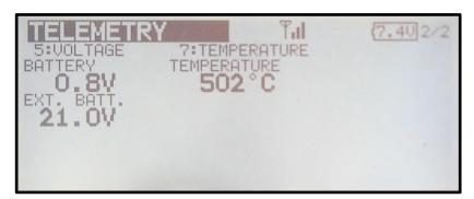
0.8V ..... Pump voltage 21.0V ........... 21% Throttle 502°C ..... EGT
