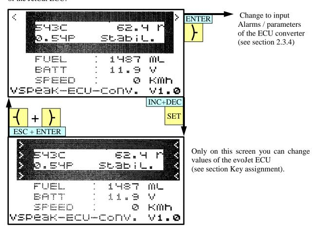
The functionality of the JetCat GSU can be mostly replicated with the HoTT buttons. For further details on the specific values please consult the manual of the JetCat ECU.
