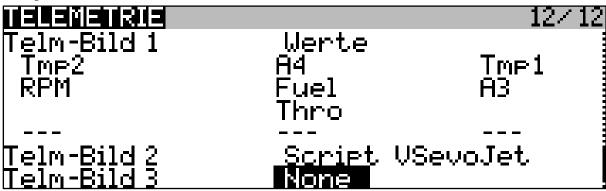
... so that the telemetry data of the VSpeak ECU converter can be displayed clearly with the corresponding status messages:
