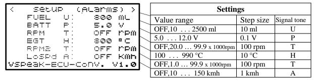
Upon delivery, the warning thresholds are set as shown in the picture.
