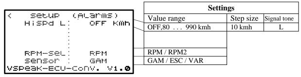
Upon delivery, the warning thresholds are set as shown in the picture. As can be seen in the table, the alarms for HiSpd can be switched OFF
