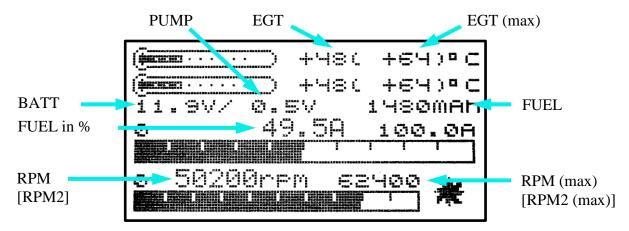
The ESC temperature display is limited to 235  $^{\circ}$  C, so the turbine jet temperature is shown divided by 10, or the other way around: 48  $^{\circ}$  C in the display corresponds to 480 ... 489  $^{\circ}$  C.
