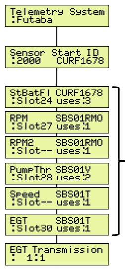
Here the sensor start ID can be set, which is used to register the sensors of the VSpeak ECU converter on the Futaba system.
