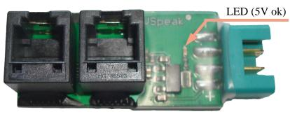
The Programming adapter is the power supply of the GSU and the VSpeak converter from a 2-3 cell LiPo / LiFe / LiIo battery (for example receiver or turbine battery).
