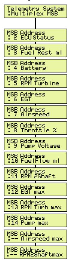
For the Multiplex Sensor Bus (MSB) a variety of settings in VSpeak ECU converter using the Programming adapter + JetCat GSU can be made.
