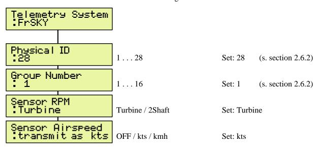
The parameter "Sensor Airspeed" is used to set how the speed value is to be transmitted via S.Port telemetry. The value supplied by the JetCat ECU in kmh must be transmitted as kts so that the speed value is displayed correctly in kmh in the taranis. The speed transmission can be deactivated with the VSpeak ECU converter - e.g. if a FrSKY speed sensor has been installed in the model.
