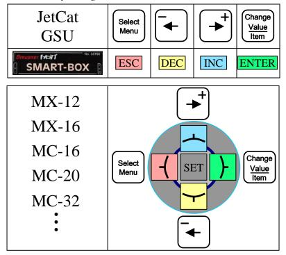
Unlike the JetCat GSU, the HoTT buttons for the functions "Select Menu" and "Change Value / Item" have a switched effect, means, one times pushed the button activates the function - one times again deactivates the function.
