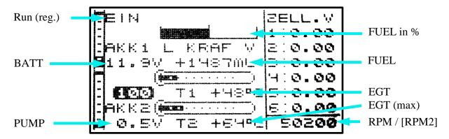
"EIN" indicates that the turbine is in the "RUN (reg.)", "SpeedCtrl" or "Rpm2Ctrl" status.
