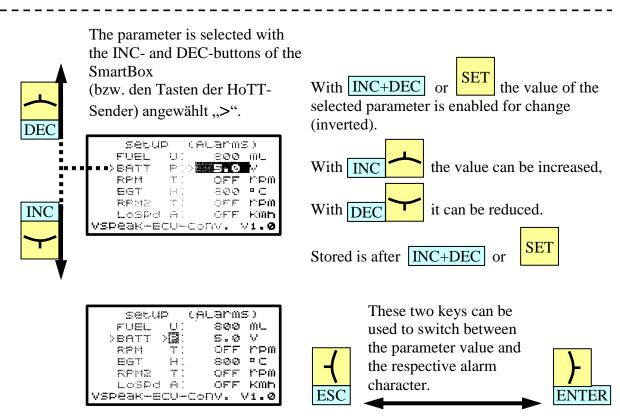
If the alarm code is activated (inverse displayed), the alarm message assigned to the respective letter is announced, which can be different for the 3 types of types GAM / ESC and VAR.
