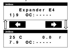
If the VSpeak ECU Converter is connected to an Expander or Centralbox and the ECU Converter display is activated with the Right button, the only way back to the expander menu is pressing the Left button (more then 3 sec).
