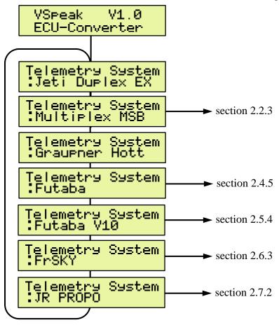
With Jeti and HoTT, all other settings can be made directly from the transmitter. For all other remote control systems further specific settings can be made (follow the respective section). With the "Limits" button you can switch to the "Global" parameters (see next page). Press the button "Select Menu" returns to the "Telemetry System Selection".
