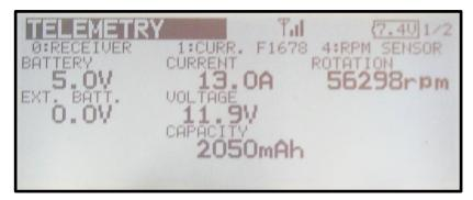
13.0A..... Run (reg.) 11.9V ..... Turbine battery 2050mAh ..... 2050ml remaining Fuel 56298rpm..... Turbine Speed
