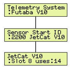
Here the sensor start ID can be set, which is used to register the sensor on the Futaba system. In the case of multi-trubine models, different values must be set here.
