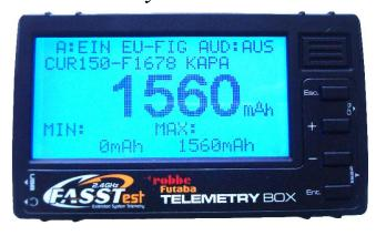
On the Telemetry Box, the data of the VSpeak ECU converter can also be displayed (in the picture e.g. fuel consumption 1560ml) and alarms corresponding section 2.4.4 are generated:
