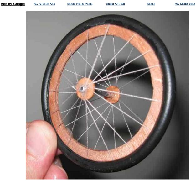
Build your own thread RC plane plan spoke wheels - no special tools required
