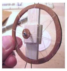
Spoke wheel axle jig pinned in place with eight thread spokes
