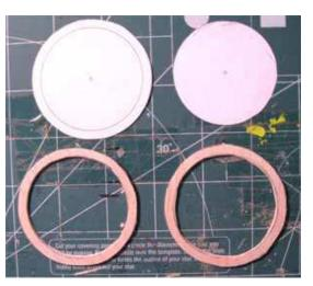
Two 1/16" balsa spoke wheel blanks - glue cross grain for strength
