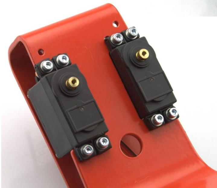
*The servos are mounted each with four cylinder head screws M3x12, four washers and four nuts.*
