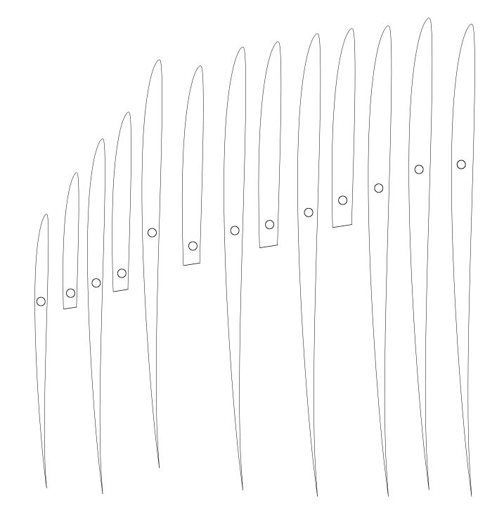
MRCSS Bug Mod 1 January 26 2013 6% thick foil .13 % Camber As per Builder's options/leading/trailing edge etc.
