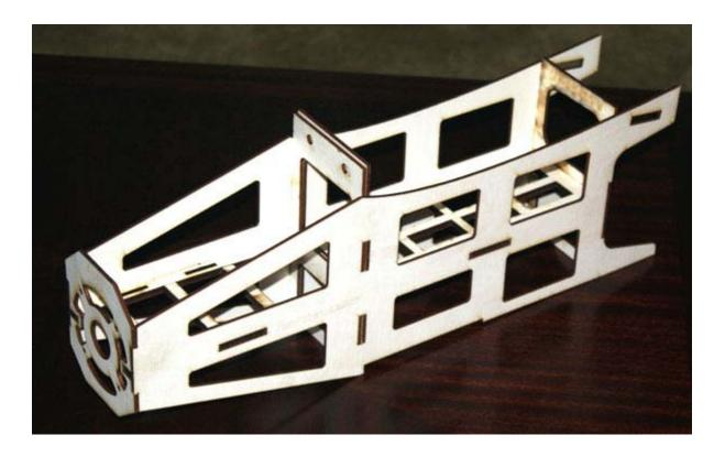
The laser-cut fuselage construction uses a snap-together tab-and-slot box, consisting of the forward fuselage doublers and several formers. These assembled to a tray for the servos, and either a battery or a fuel tank. This arrangement, besides being immensely strong, helps ensure alignment of the fuselage.
