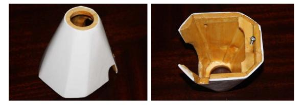
For construction methods, refer to articles appearing in Model Aviation and other publications. The cowl was finished with Hangar 9 UltraCote as was the rest of the model.
