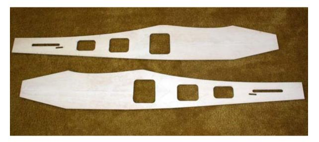
Because of available sheet-balsa sizes, the fuselage sides are assembled in three pieces. Use suitably matched 1/8 balsa sheet material. Secure the fuselage plans to the building board. Affix a translucent transfer medium, such as shelf paper or vellum over it, and carefully trace the three-piece fuselage side outlines. Transfer the traced images to the balsa sheets and make two copies of each section.
