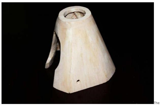
cowl is a simple structure made from 3/8 balsa sheet, and is specific to the power plant used. A chin scoop should be present for an electric-powered model to ensure proper motor cooling.
