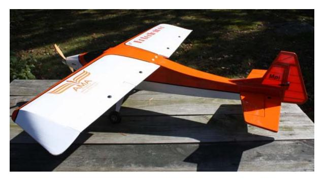
A further option is the extended wing. If you are looking for a model with a wing loading of less than 20 ounces per square foot, the extended wing set provides this. The standard wing is just the ticket for spirited sport flying, while the lighter loading of the extended wing might be better for those with 3-D aspirations, or those desiring a slower-flying model.
