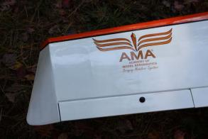
Using water slide decal paper and my inkjet printer, I made the AMA logo seen on the left wing, and the name I gave the model on the right wing. The printer ink is not waterproof, so I applied several coats of clear Krylon to seal the decals. I also sealed the edges after application with clear Krylon applied with a small brush.
