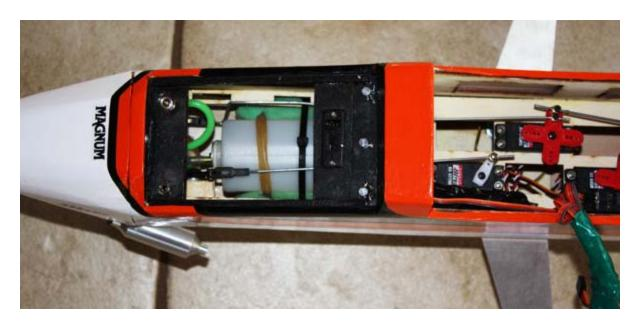
The inclusion of the hatch on my glow-powered EnterTrainer prompted a few additions. The inverted engine makes it awkward to connect the glow plug, and the cowl prevents easy access to the fuel tubing.
