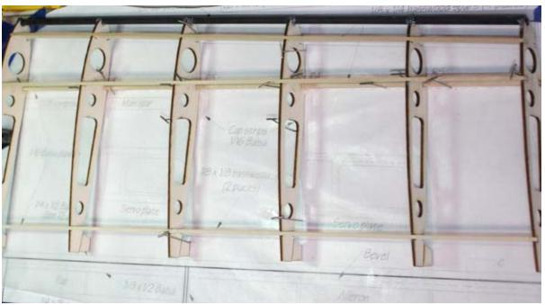
The following instructions apply to both wings and both wing sets. Secure the centermost top spar to the plans. Using it as a guide, use medium CA to adhere the ribs. Ensure that they are square, and that the break-off stubs are flat on the building board. When complete, assemble the bottom  $1/8 \times 1/4$  basswood front and center spars, as well as the 1/8-inch square rear spar to the ribs. Cut the .317 diameter composite LE to size and snap it in place. Use medium CA to secure it.
