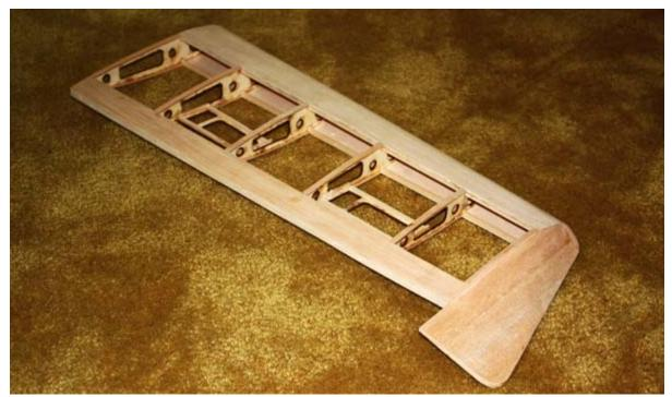
The wingtip parts are cut according to the detail on the upper right of the wing and empennage plan. They are assembled as shown, giving the tips a 1-inch droop. They should be planked entirely with 1/32 balsa for strength. When complete, bond them to the wings using medium CA.
