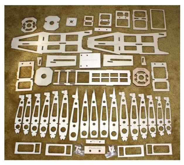
Depending on whether you will be using glow power or an electric system, you will need to select which firewall and former F2 to use. Those for the electric contain the necessary slots for proper cooling.
