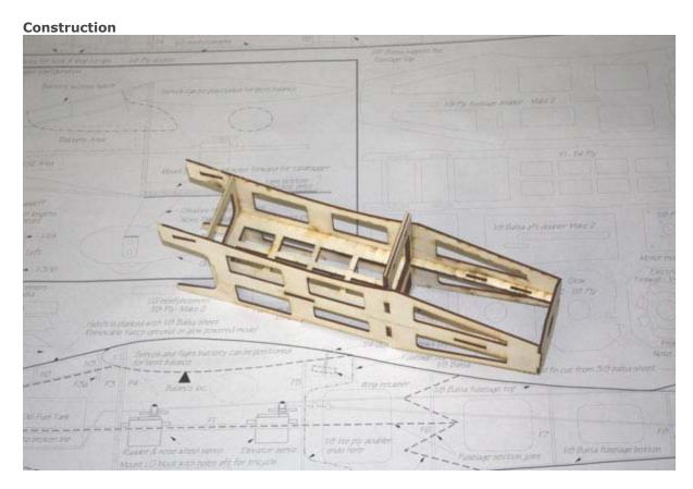
This model is for an intermediate builder, and I would not recommend it as a first construction project, because some careful carving and shaping is involved. I suggest building the fuselage first, because it is the more complex of the assemblies involved in building EnterTrainer.
