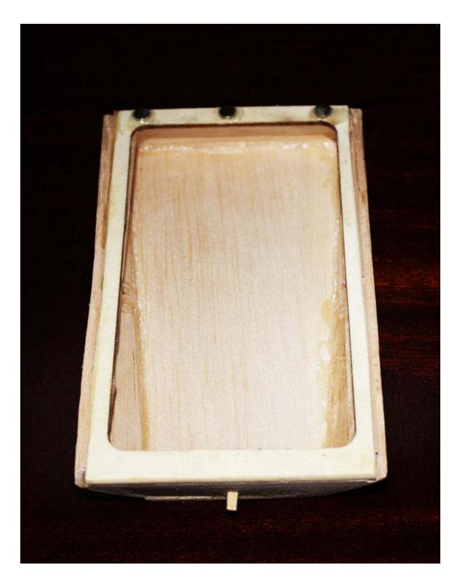
The hatch and adjacent structures require care in assembly. Refer to the plans and photos as a guide in order to obtain a proper fit. Use a file or a sanding block to bevel the firewall/F2 and the F3/F4 assemblies, ensuring a smooth transition between the firewall and the hatch.
