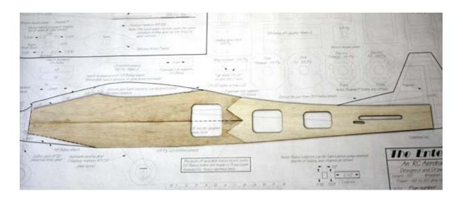
With the fuselage side sections available, cover the plans with waxed paper and pin the balsa sections for one side in position over it. Use medium CA adhesive to bond the sections together. Put another layer of waxed paper over the completed fuselage side and repeat the procedure with the remaining balsa sections. This method ensures that the sides come out identical and true to the plans.
