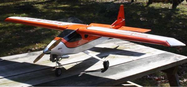
The airplane's configuration is that of the familiar stick model, with the wings and empennage altered to suit the purpose of this design—that of a stable platform from which to learn the basics of RC model aerobatics.
