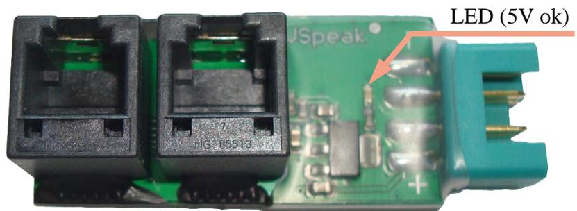
The Programming adapter is the power supply of the GSU and the VSpeak converter from a 2-3 cell LiPo / LiFe / LiIo battery (for example receiver or turbine battery).
