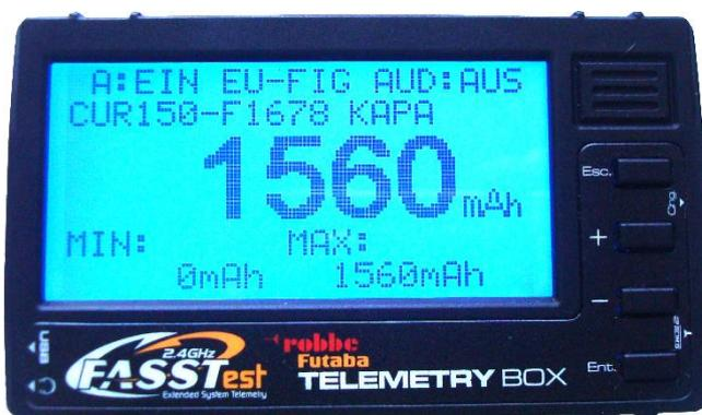
On the Telemetry Box, the data of the VSpeak ECU converter can also be displayed (in the picture e.g. fuel consumption 1560ml) and alarms corresponding section 2.4.4 are generated:
