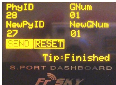
For this purpose, the Telemetry port of the VSpeak ECU converter must be connected with a V cable and a receiver battery to the FrSky DASHBOARD. Furthermore, the ECU converter must be connected to the powered JetCat ECU or with the Programming adapter
