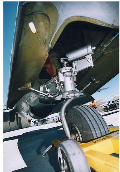
Tailwheel detail, I had to crawl on the ground and use a flash to get this shot. Notice the color of the interior and scoop detail in front of tailwheel.
