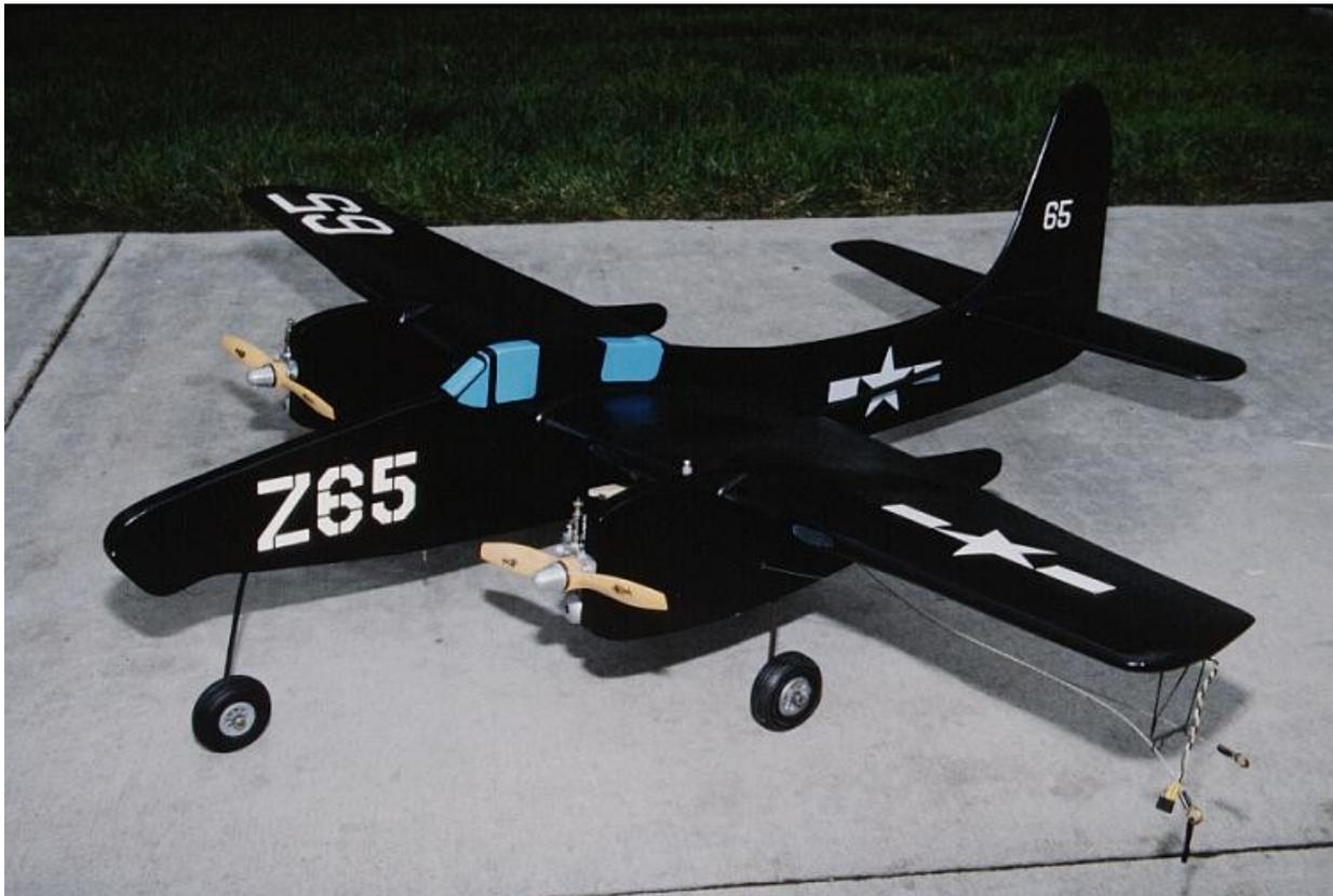
**Photograph 10.1** - Author's scratch built 41" span Profile Scale Grumman F7F-3N Tigercat with OS-15FP's for power. Single channel electronic controls buried in wing, nacelle, and fuselage. Notice electronic hookup connector and leadout guide at wingtip. On-Off switch can be see directly below the Z65 on the fuselage. This model weighs 3 lbs and has a foam wing.
