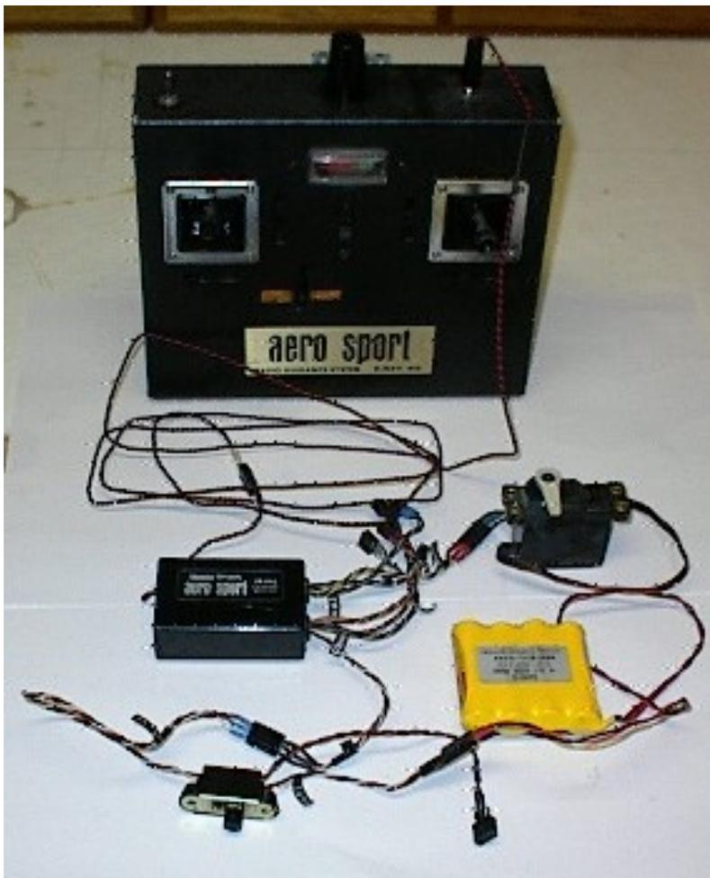
This is a typical radio control unit that has been converted for CL use. The wire plugged into the top of the transmitter carries the signal and ground out to the two flying lines. This unit happens to be a 6-channel unit with only one servo shown.
