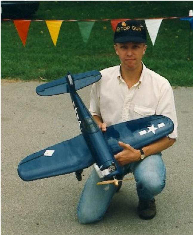
**Plate #10-** Fred Cronenwett with his 36" span Sterling Corsair in 1990, Single channel controls, monokote for covering. This model was powered with an OS-25FP. This model is so small the only thing that could be installed without making the model too heavy to fly was a throttle servo. The model weighed 3 lbs and flew on 52 foot lines
