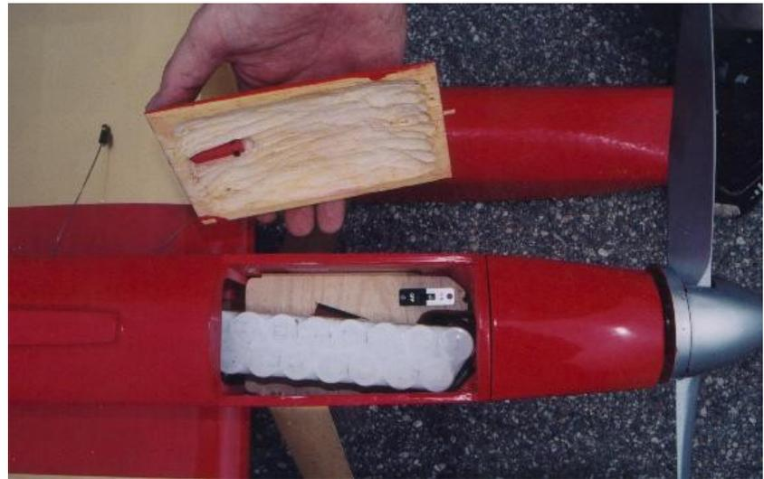
This is a SR battery pack (18 cells) that is held in place with Velcro. Move the battery to correct any CG problems. Unless you absolutely have to, do not add any nose or tail weight on an electric powered model to correct the CG location, move the battery as needed.
