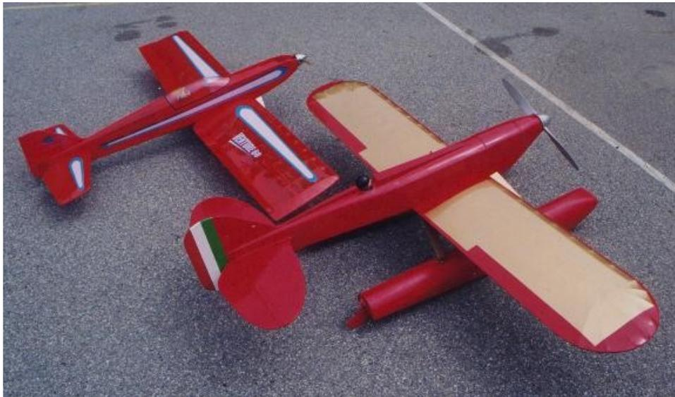
**Photograph 7.1** - Grant Hiestand's Venture 60 electric powered airplanes, the stock Venture 60 is on the left, the highly modified version was kit bashed to look like a Macchi MC-72 Schniieder cup Air Racer. Both models are powered with an Astroflight 40 electric motor and use electronic controls.
