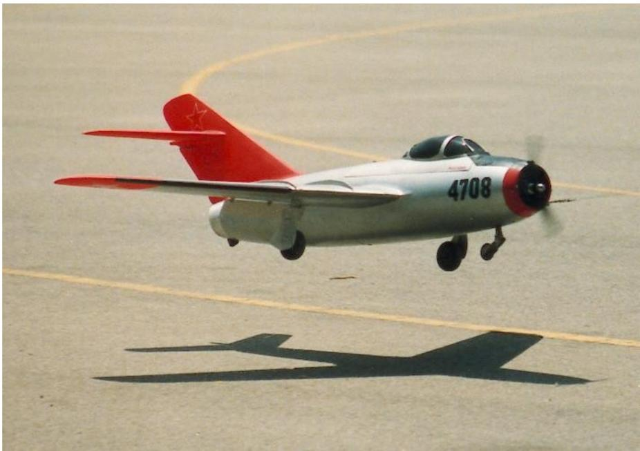
**Plate #12-** Flown by Merle Mohring, this Mig 15 was fast and a challenge to fly. You can see here is has a prop in the nose. You can't see the tuned pipe that runs thru the fuselage.
