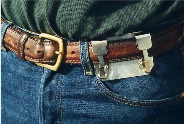
**Photograph 5.6** - Grant Hiestand's and Fred Cronenwett's solution for hanging the transmitter. Simple device was made from two key clips, pop rivets and aluminum. The metal bar on the transmitter clips on as shown.
