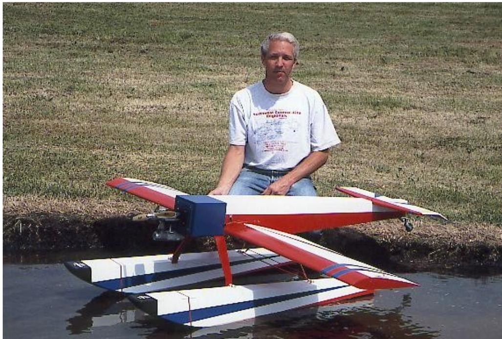
**Plate #6-** Fred Cronenwett with his scratch built Camera plane on floats. This model can be flown from water or land. 80" span, shown here with an ST-90, but has since been replaced with an OS-91 four stroke. DSC electronic controls. This is a wonderful test aircraft for motors, electronics, camera platform and other features.
