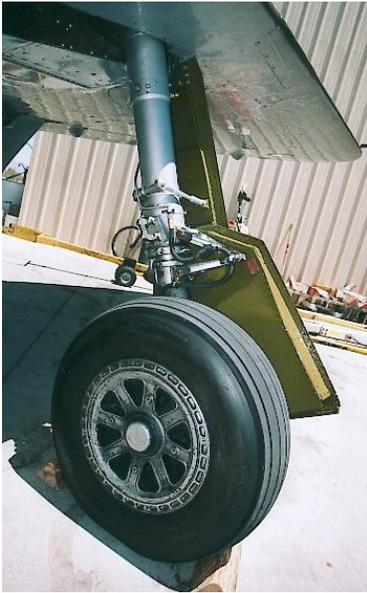
Inboard sides of landing gear leg showing wheel, strut and door detail
