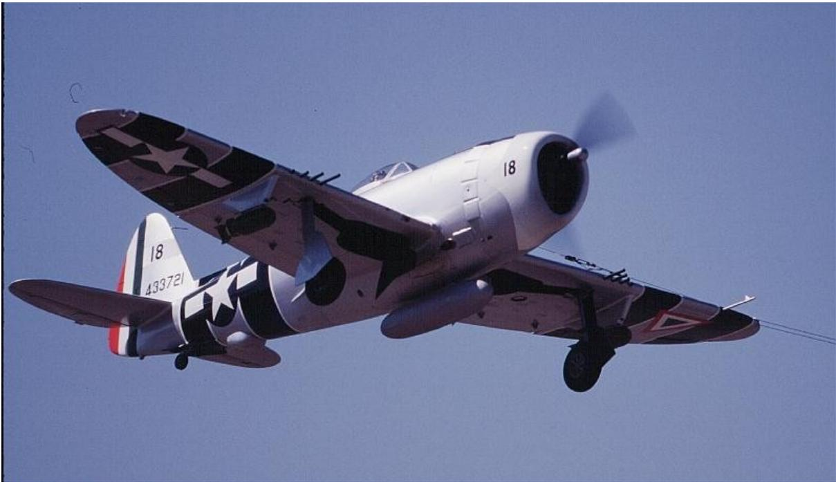
**Plate #7-** Lynn Boss's P-47 Bubble top Thunderbolt from the Top Flite gold edition kit. This model uses DSC controls for retractable landing gear, flaps, throttle, tank & bomb drop and steerable tailwheel. This is a precision scale model that is powered with an OS-90 four stroke.
