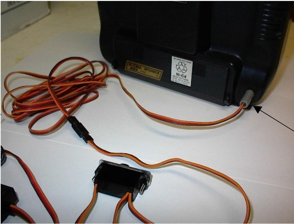
Inspect the wire underneath this cover to make sure the wires don't short out. This can happen as the cord gets twisted during daily use. If the wires short out here the system will be inoperable.
