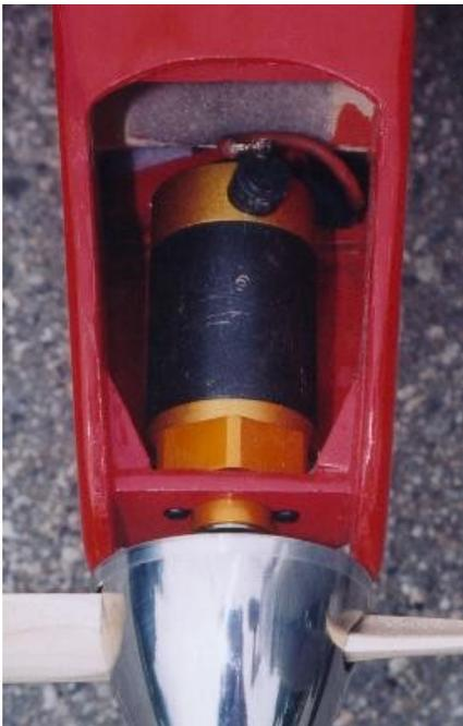
**Photograph 7.2** - This is how Grant installed the Astroflight Geared 40 in the stock Venture 60.
