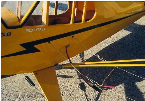
**Photograph 14.2** - Notice location of the bellcrank and landing gear location.
