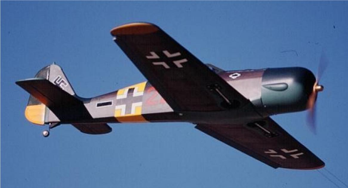
**Photograph 11.3** - Author's FW-190 from the Great Planes Almost Ready to Fly kit. This kit is no longer available. This model features flaps, bomb drop, throttle and retractable landing gear. Notice that the ailerons intended for radio control were used as flaps. This photo was taken when the model was being tested with an electric motor before the bomb drop unit and a .46 sized glow engine were installed.
