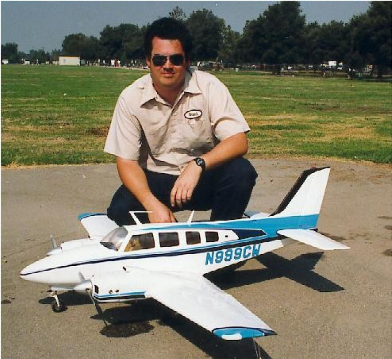
**Plate #9-** Grant Hiestand with his scratch built Beechcraft Baron 58 from Royal plans. This model featured retractable landing gear, flaps and throttle with multi-channel electronic controls. A pair of twin Fox .40 sized glow motors was used for power. The model spans 72” and weighed 11 lbs. Grant found a Baron at the local airport, took pictures and duplicated the paint scheme on his model. This model was flown in Sport Scale.
