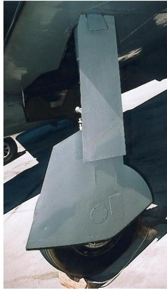
Outboard side of landing gear leg shows door detail
