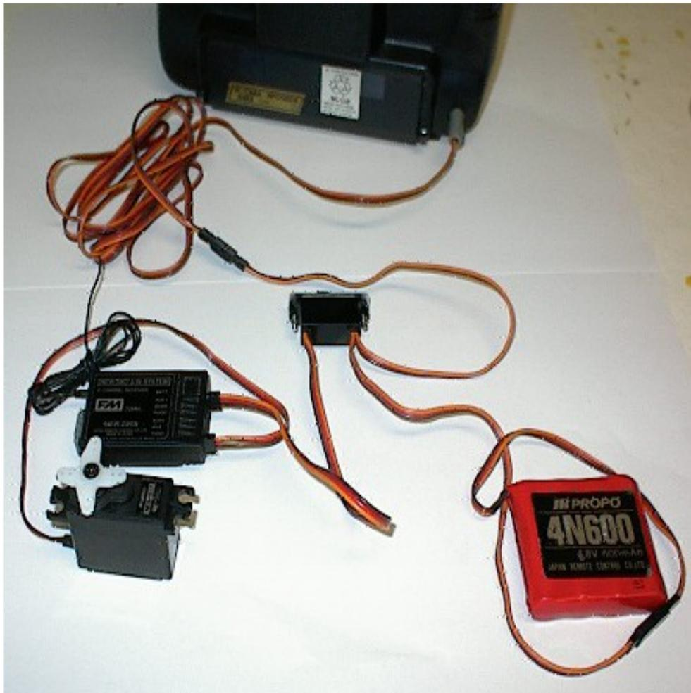
**Photograph 5.1** - Shown here with one servo plugged into receiver and deluxe switch harness, this system will not work with standard switch harness
