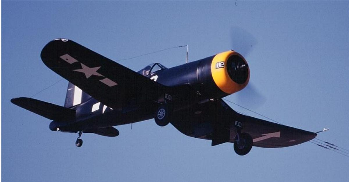
**Photograph 11.2** - Lynn Boss's F4U corsair built from the Royal Corsair SR kit that was intended and labeled as a Radio Control Kit. This model spans 63" and is powered with an OS-90 four stroke. This particular model uses a 3-line bellcrank for throttle control and features bomb drop with down elevator.
