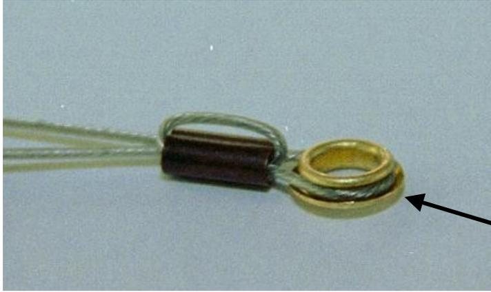
Pull the wire loop around the brass thimble tight as shown. Crimp the tube with standard pliers to keep the loops from moving. This style of line assembly has been pulled tested to 80 lbs during competition without failure. The brass Thimble shown is from a Sig package but is also available from Brodak Manufacturing.
