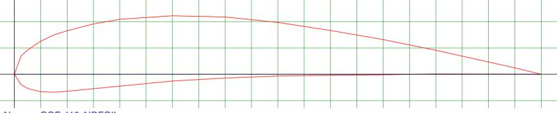
Name = GOE 418 AIRFOIL Chord = 200mm Radius = 0mm Thickness = 100% Origin = 0% Pitch = 0°
