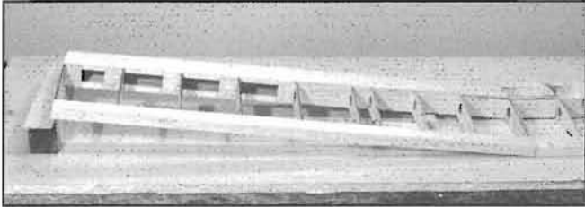
Join the wing panels using a 2-1/4" block to raise the tip. Don't forget to build the washout into the second panel.
