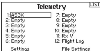
1. In the telemetry screen in one of the empty positions select AS3X and activate the Display. This will activate the AS3X Gain menu in the Function List.
