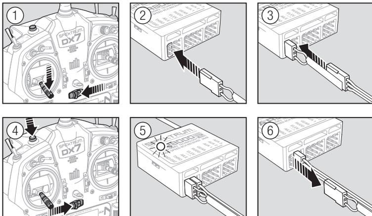
1. Lower throttle to the lowest position and make sure the transmitter is powered off.
