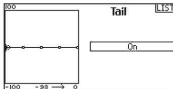
Always enable Expo when using a standard rotating-arm servo. The Expo delivers linear movement of the swashplate from a standard rotary servo. When Expo is inhibited, the arm on a rotary servo moves on a curved path with decreased swashplate movement at the extremes of the servo arm travel.
