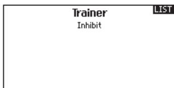
**CAUTION:** Select Inhibit in the Trainer menu when you aren't using the wireless trainer function. Failure to select Inhibit may result in loss of control of the aircraft.
