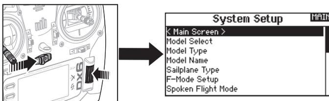
You can also enter the System Setup from the Function list without turning the transmitter off. A Caution screen will appear that warns that RF will be disabled (the transmitter will no longer transmit). Press YES if you are sure and want to access the System List. If you are not sure, press NO to exit to the main screen and continue operation.
