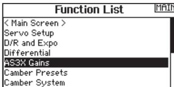
2. In the Function List Access the AS3X Gain menu. If an AS3X receiver is bound to the transmitter and the receiver and transmitter are on, live gain values will be displayed on this screen.
