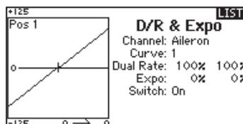
Exponential affects control response sensitivity around center but has no effect on overall travel. Positive exponential decreases the sensitivity around the center of gimbal movement.
