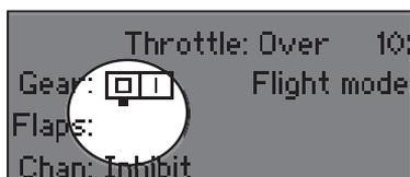
**Tip:** The tick mark below shows the current switch position. Rolling and clicking the scroll wheel turns the selected box black, indicating that the value or condition will act on that position.
