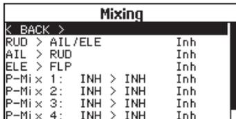
Select a channel for master and slave. Inputs for the master channel control both the master and slave channels. For example, Elevator to Flap makes elevator the master channel and flap the slave channel.
