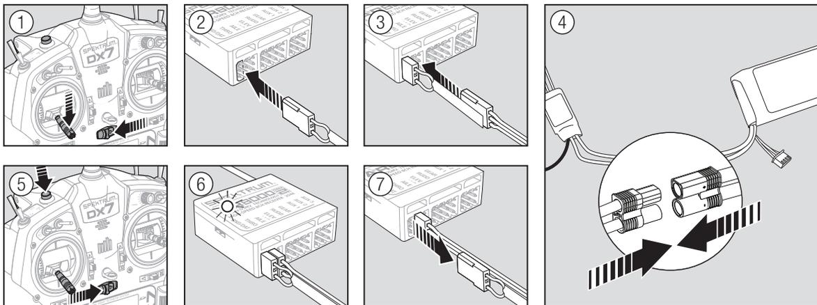
1. Lower the throttle to the lowest position and make sure the transmitter is powered off.
