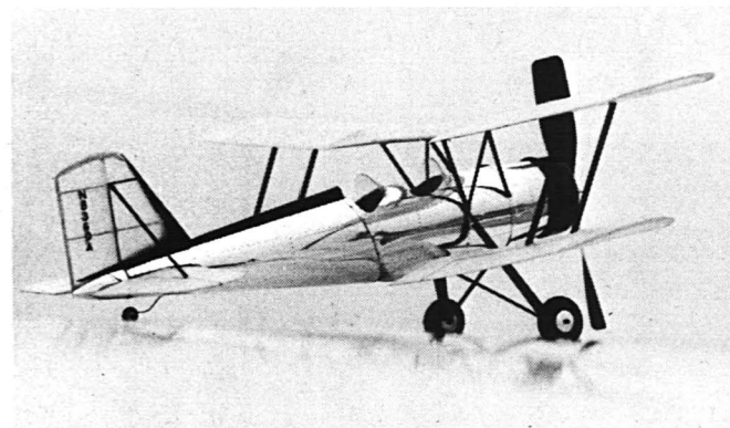
Aluminized mylar simulates metal covering. Note rivet detail on fuselage.
