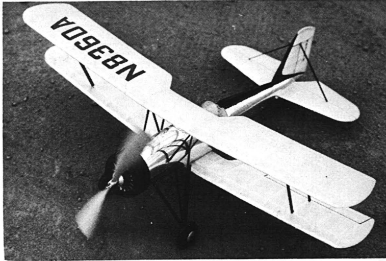
Front view with prop spinning shows effective use of metallic mylar.
