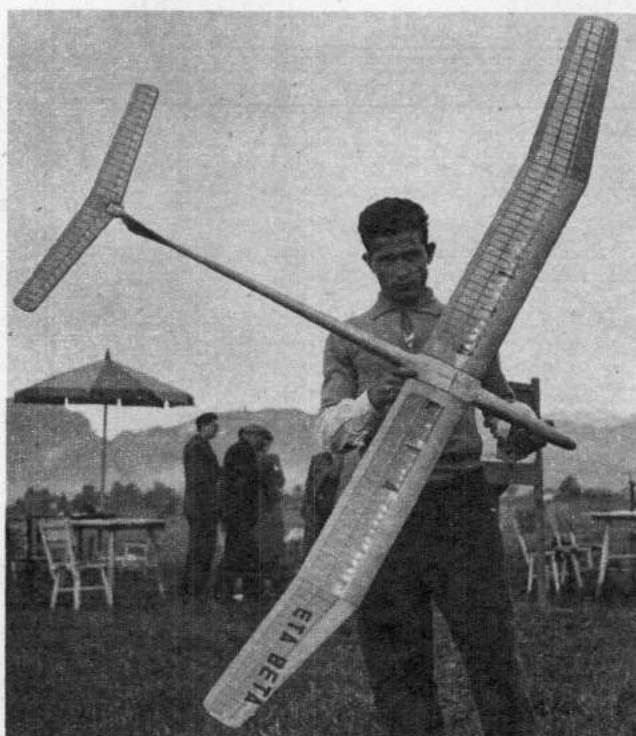
Italian "Eta Beta" entry had superb finish. Stab mount atop rudder tricky due to small hinge surface for pop-up action.
