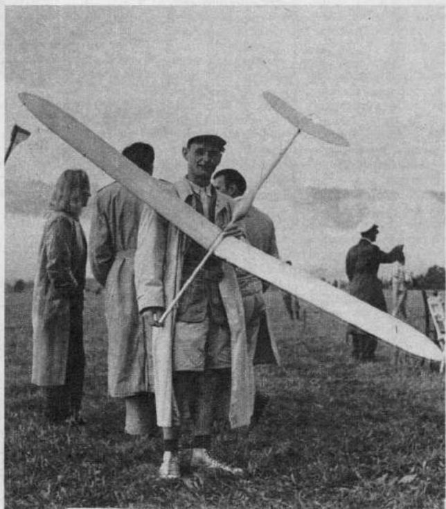
German fan; 103-inch wing. Aspect ratio 25.5 to 1; wing flexed greatly on tow. Turbulators; pod for cross section. Note raincoats.
