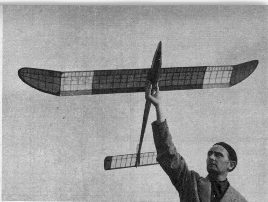
"Nordic" champion Hans Hansen of Denmark made 3 5-min. flights. Wide trailing edge on center wing panels is hinged flap to be utilized for final trim if necessary.
