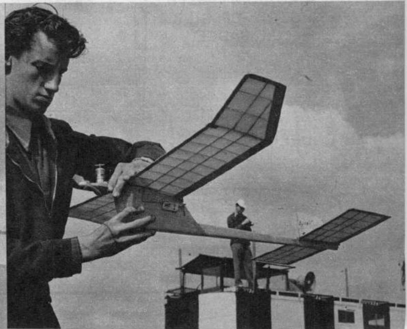
Proxy-flown Swedish entry by K. Ericssen illustrates high thrust line which finds favor overseas. Power is by E.D. 1.46 cc diesel.
