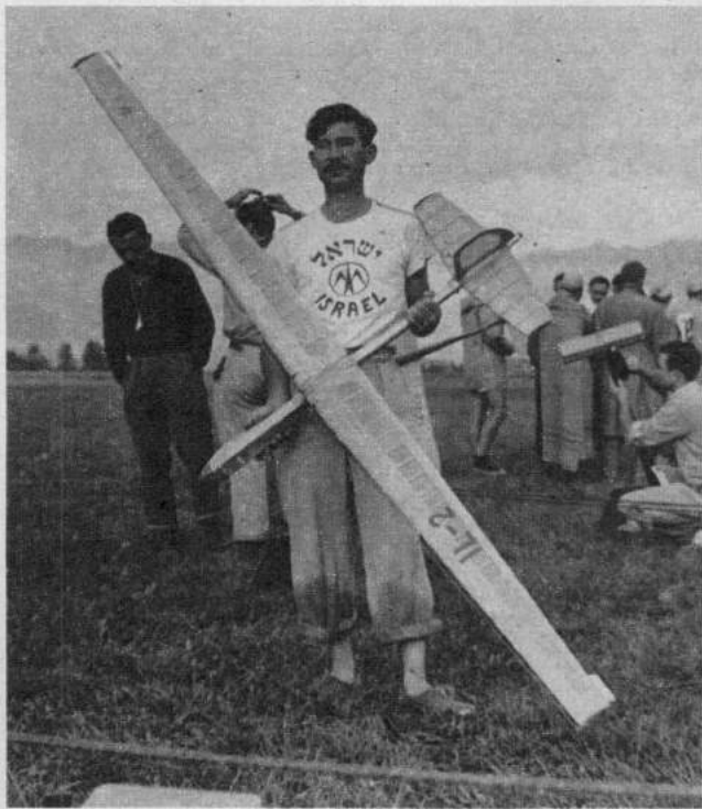
High aspect ratio entry from Israel. Flyer Fred Meir also utilized a turbulator wire on wing ahead of leading edge. Commendable fry.
