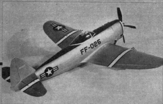
Designer Musciano found that most any engine from .13 to .35 cu. in. can be used to power your P-47. Those .19-.29 will be best.
