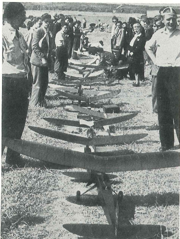
French diesel line-up during their Nationals. Significant feature of this picture is the almost universal adoption of tapered or elliptical wings.
