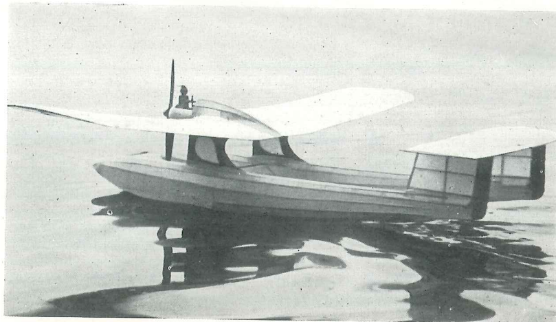
A Swiss flying-boat embodying twin hulls and "power-egg". This type of experimental model is particularly suited to diesel power for no matter how many duckings it receives it will go on flying until the covering is soaked off by constant immersion!
