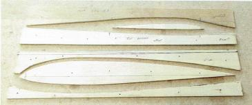
Templates for the Spitfire cores, with the tip template made the same size as the root
