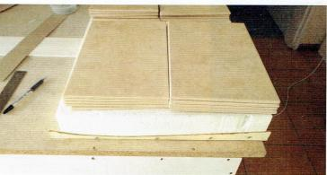
Foam on the workbench ready to be cut. The balsa sheet is in the middle of the block and the tiles help bend the foam
