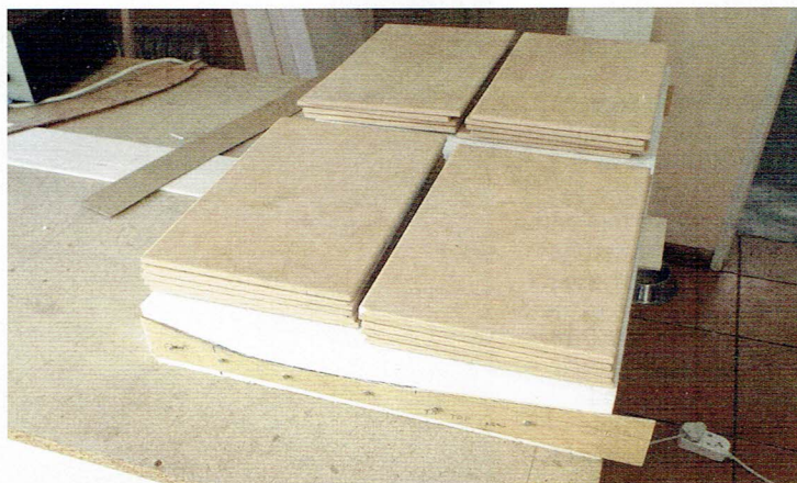
Getting ready to cut the upper surfaces, marking the thickness needed by using the original tip template. Measure three times and cut once. Do not ask how I know!
