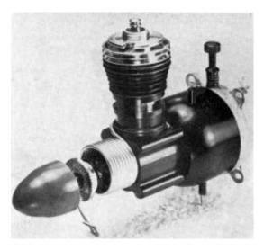
needle valve. The fuel inlet to this is through an internal tee, integral with the backplate, which is fitted with a short length of fuel tube. The tube is lined with a fine spiral wire spring to prevent kiriking. Air is fed to the engine from a channel in the rear face of the backplate, through a gauze dust filter and, on picking up fuel from a jet hole below the needle-valve, the resultant fuel-air mixture is conveyed forward through a divergent induction tube in the centre of the tank.
