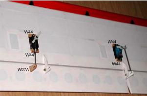
**10.** If required, glue optional plywood servo beds(W44). You may use a servo reverser when you connect flap servos with Y-harness, if not, install optional flap horn(W27A).
