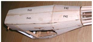
18. Glue fuselage lower panels(F41, F42).
