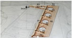
**5.** Pin the sheet(R6) on the plan and glue frames(R1-R5,R7).
