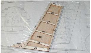
1. Lay the waxed paper or PVC film over the plan. Pin the vertical fin sheets(V10-V11) and frames(V1-V9). Glue them with thin CA.
