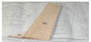
**2.** Remove pins and glue the sheets(V10, V11) with thick CA.
