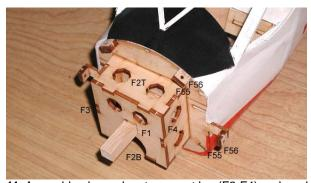
**11.** Assemble plywood motor mount box(F2-F4) and cowl mounts(F55, F56). Make sure to pay attention to bulkhead F1 the numbers should be facing forward.
