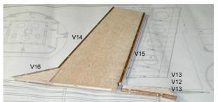
**3.** Glue the leading and trailing edges(V14-V16) with thick CA. Glue stabilizer bed(V12, V13) together.
