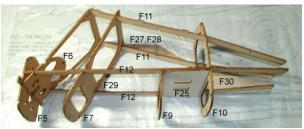
**3.** Lay right side parts(F27, F28, F29, F30) on the plan and temporary assemble right longerons(F11, F12), bulkheads(F5, F6, F7, F9, F10) and servo bed(F25). And then, install left longerons(F11, F12).
