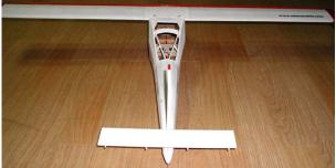
6. Glue stabilizer and vertical fin to the fuselage with thick CA. (Horizontal tail must be paralleled with wing and vertical fin must be at right angle to horizontal tail. Wings must be installed temporarily to align them.)
