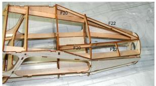
7. Install rear cockpit frames(F20, F22). Now glue all the parts together with thin CA. And then, **Apply** thick CA glue at each joints for reinforcing.
