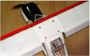
29. Assemble wing and fix with wingbolts.
