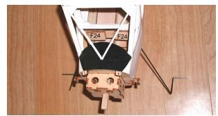
13. Glue landing gear retainer(F24).
