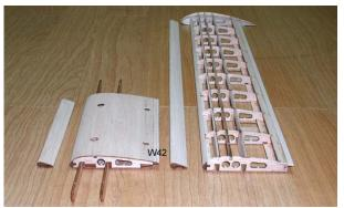
**18.** Glue center trailing edge(W17) with thick CA. **Apply thick CA glue at each joints for reinforcing.** And then, carefully sand surfaces.
