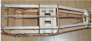
11. Glue plywood servo rails(F26).
