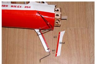
14. Assemble dummy landing gear with silicon tubes, holders(H1) and landing gear struts.
