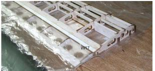
**17.** Glue trailing edge(W17) with thick CA. Refer to the wing section on the drawing and use cardboard to make a gap.
