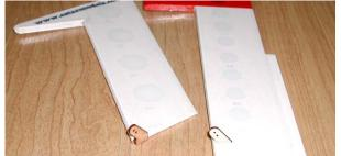
**16.** Install and glue elevator and rudder plywood horns. Apply thin CA to the horns for reinforcing.
