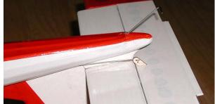
18. Insert elevator pushrod to the horn and then glue hinges with small amount of thin CA.
