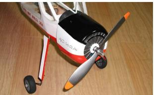
**28.** Paint and assemble cowl with 2mm screws and fix propeller.
