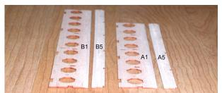
**6.** Prepare aileron and flap parts(A1, A5, B1, B5) and sand trailing edges.
