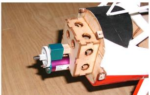
**15.** Install motor and gearbox.
