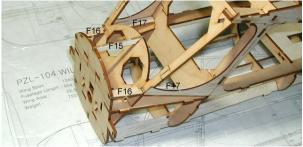
**6.** Install turtle deck frames(F15-F17). Pins and glues are not required in this step.
