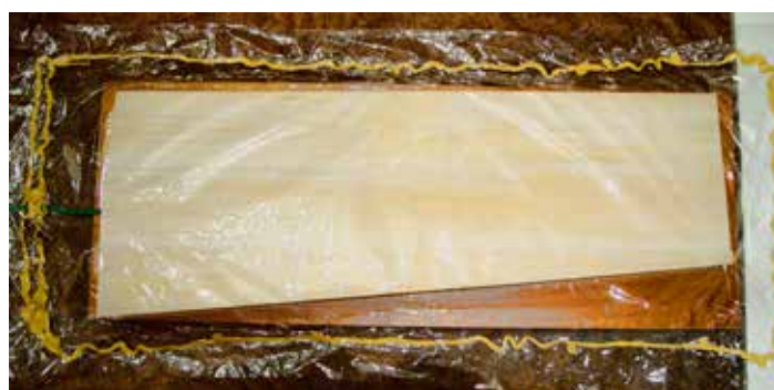
The two wing parts are moulded separately.
