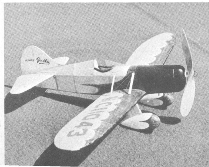
Hand-carved balsa propeller adds considerably to flight performance.
