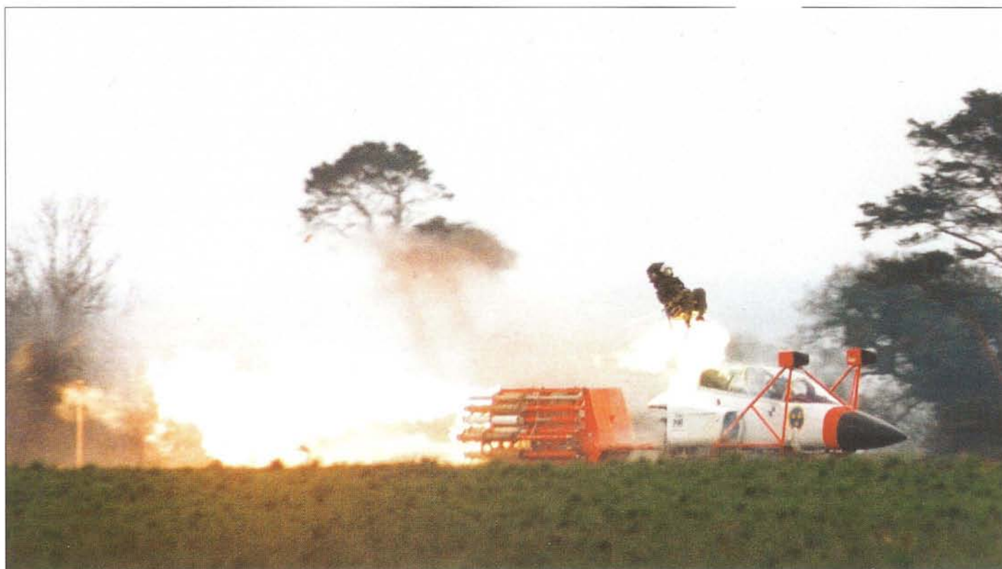
The two-seater cockpit/forward fuselage during a test ejection in 1995. Note how the pusher rockets are in full burn to propel the sled down the track at speed.
