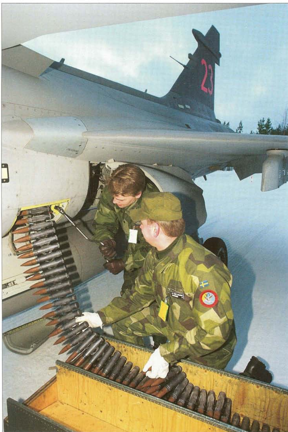
Not only the aircraft but also the ground crew have to be able to work under harsh circumstances. Here, two conscripts are rearming the Gripen's BK27 internal cannon.
