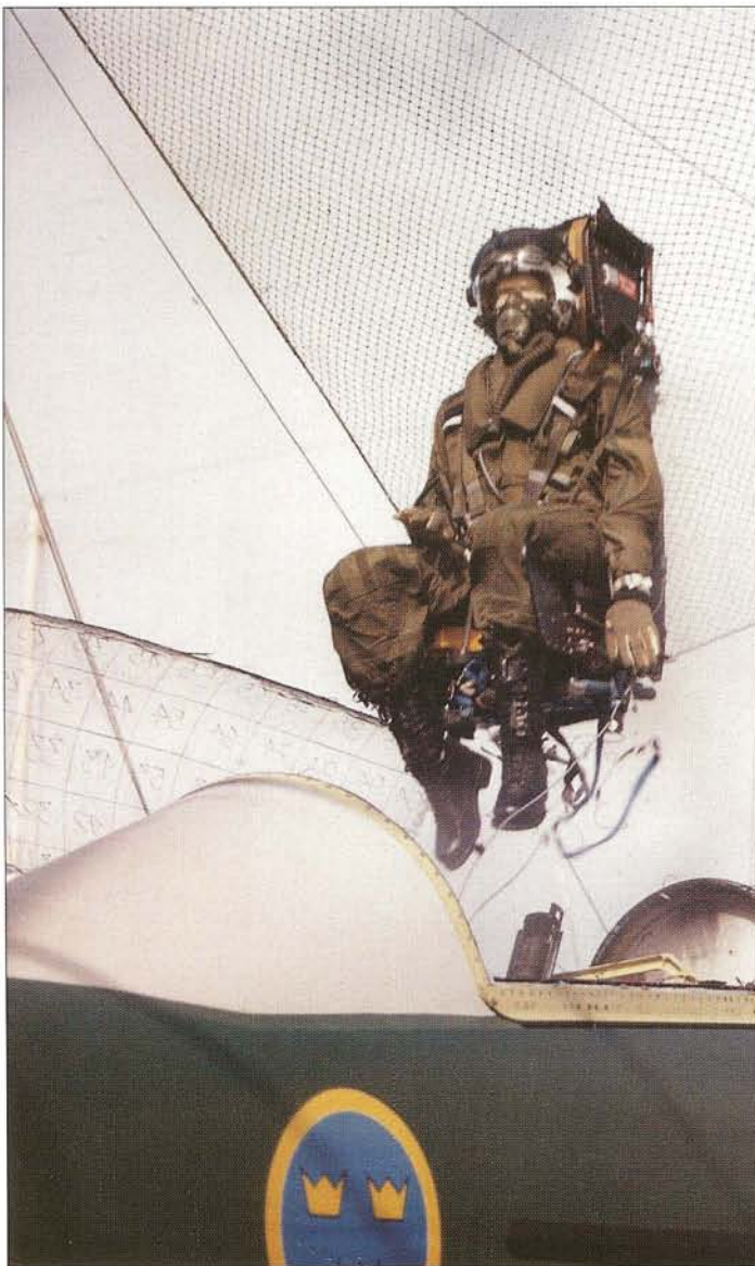
Left: A Martin Baker Mk.S10LS ejection seat undergoing a zero-zero test firing in June 1985.
