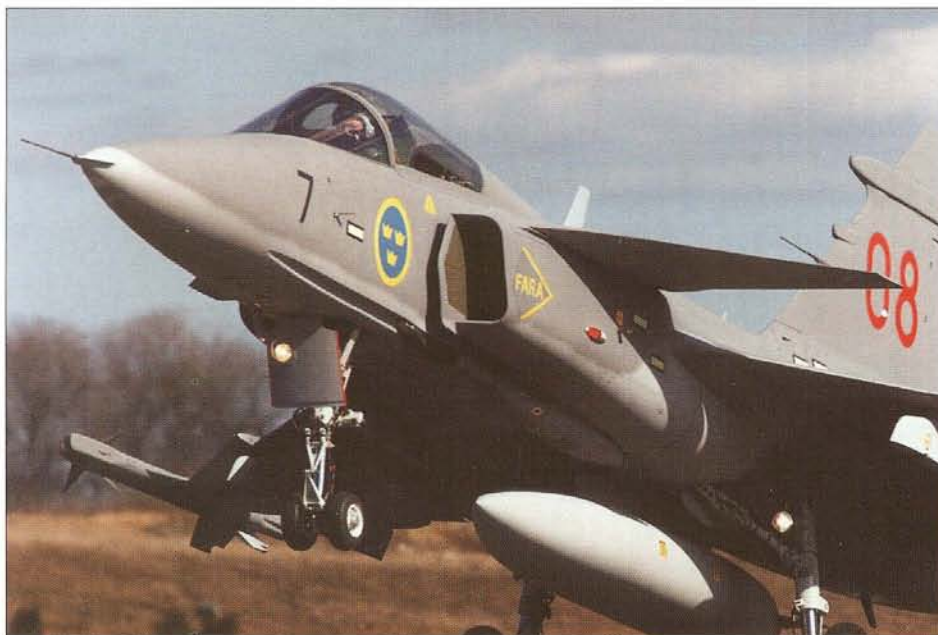
This close-up view of JAS 39A 39108 on take-off illustrates the width of the foreplane canards. The aircraft was the first to fly with a new low-pivot control stick.
