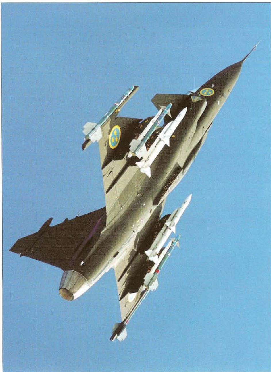
All kinds of stores were carried to test the Manoeuvre Load Limiter before the actual high 'alpha' testing was initiated.
