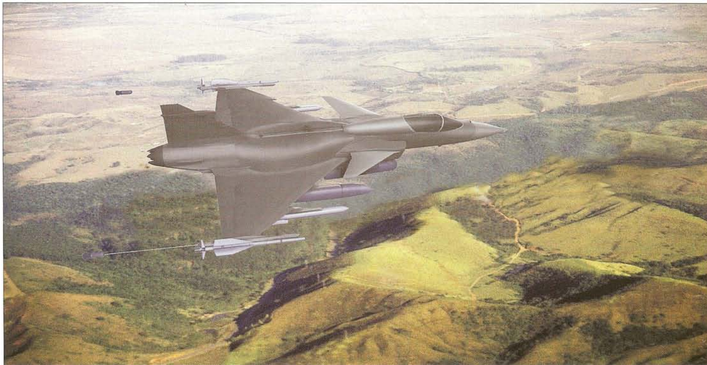
Above: Large conformal fuel tanks were one of the obvious physical additions to the next-generation Gripen proposed for 2010.
