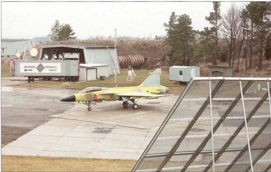
One of the prototype Gripens undergoing microwave testing in 1992.
