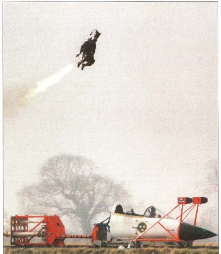
Left: A Martin Baker Mk.S10LS ejection seat undergoing a zero-zero test firing in June 1985.
