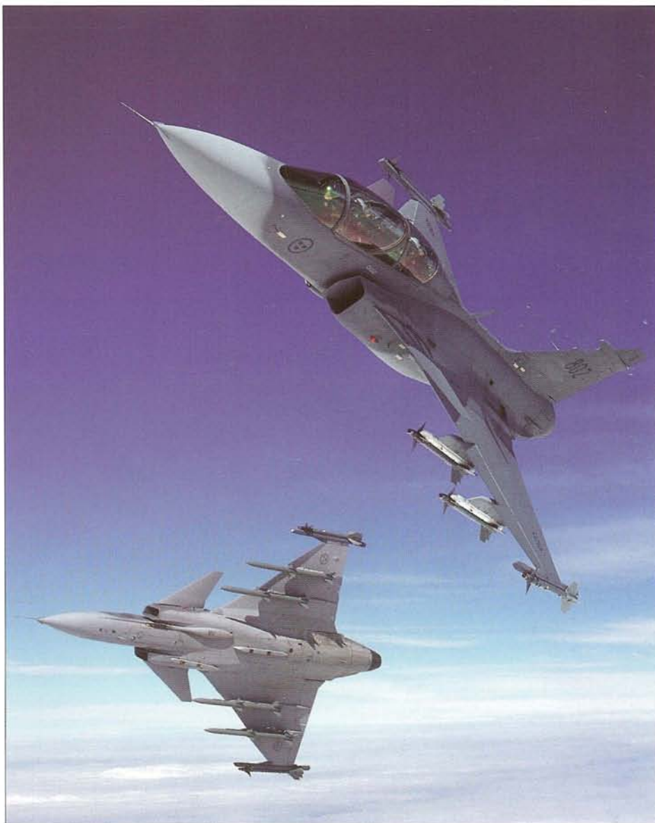
JAS 39A 39145 banks away to reveal the offset BK27 cannon pod and four Rb99 AMRAAMs on the underwing pylons, while JAS 39B 39802 displays an alternative AAM configuration of six Rb99 Sidewinders.
