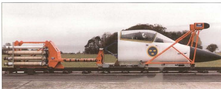
The airbag for the rear cockpit of the JAS 39B/D Gripen undergoing test inflations in 1995.
