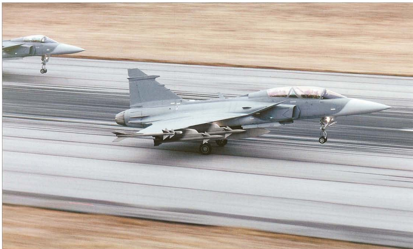
The Israeli Rafael Python 4 ASRAAM and the South African R-Darter on the Gripen; a weapon load configuration under test but not only for the South African Air Force.
