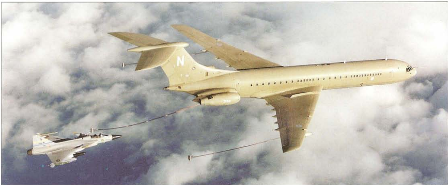
Above: Prototype 39-4 was used for the initial in-flight refuelling in November 1998 with a VC10 K.4 tanker over the Irish Sea.
