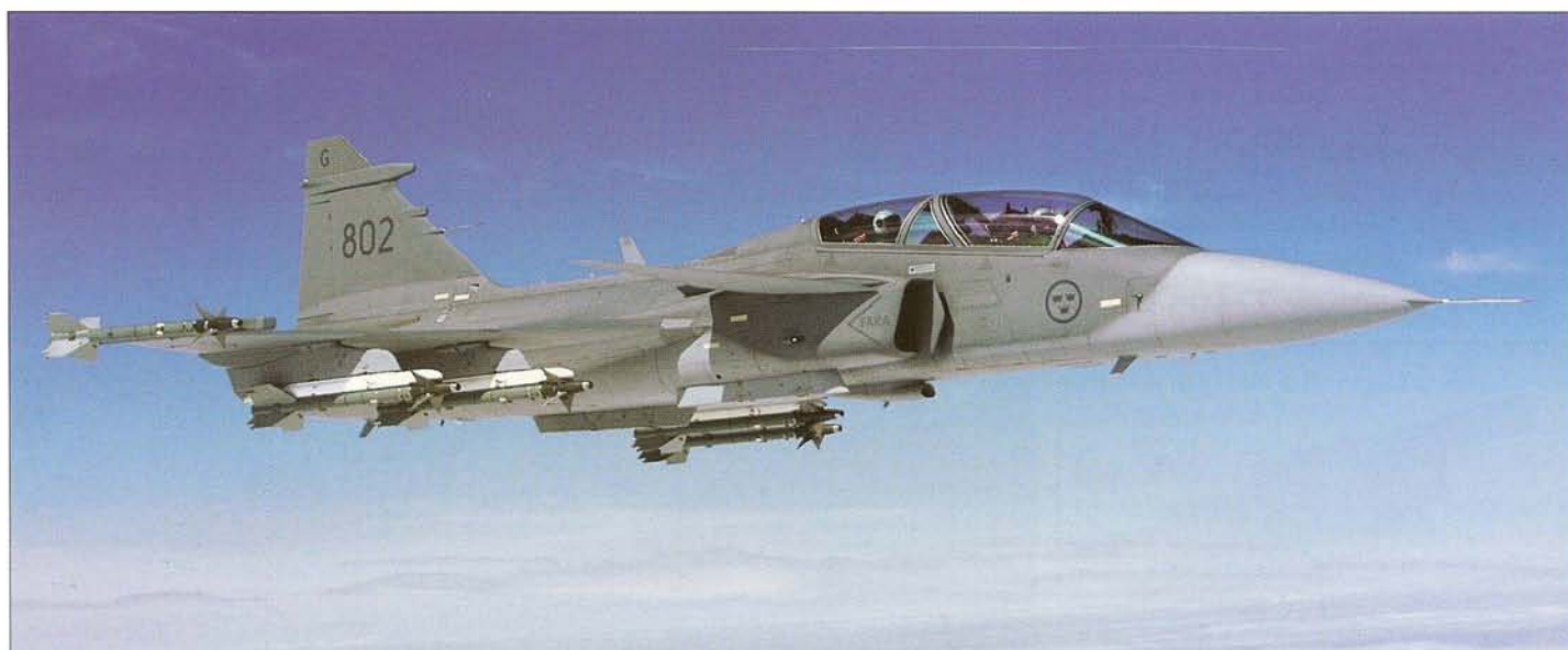
Below: Besides acting as a 'battlefield manager' the JAS 39B two-seater can actually take an active part in any conflict, as illustrated by 39802 and its weapon load of six Rb99 Sidewinder AAMs for close-in air combat.
