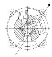
When timing ring is set correctly, daylight can be seen through inlet/exhaust ports as shown.
