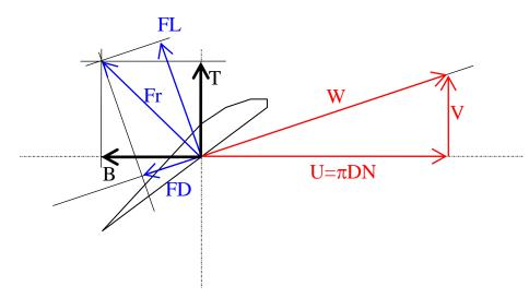
The blade is moving tangentially with a velocity U and axially with a velocity V. An aerodynamic force Fr is thus created on the blade. This force could be decomposed into a thrust T and braking force B. The blade input power is then a product of the tangential velocity and the braking force while the blade useful power is the product of the thrust and the axial velocity.
