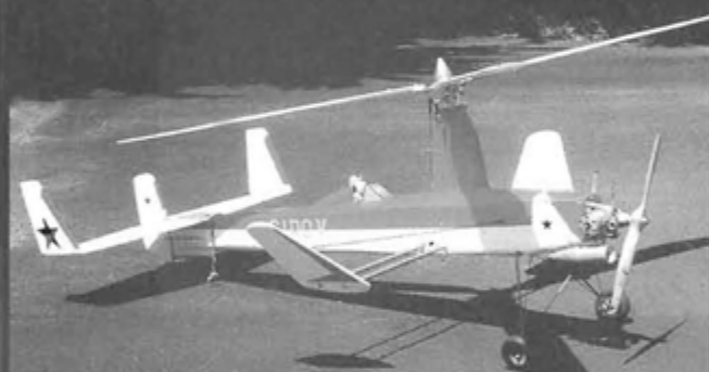
To determine if a "wing separator" had any effect on performance, the "wing" was eliminated and stability was as good or better. The "wing" apparently offered little help in other respects.
