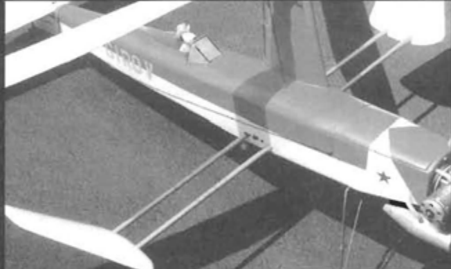
For our test, "winglets" were used as forward vertical stabilizers. Rod separators are "arrow shafts."
