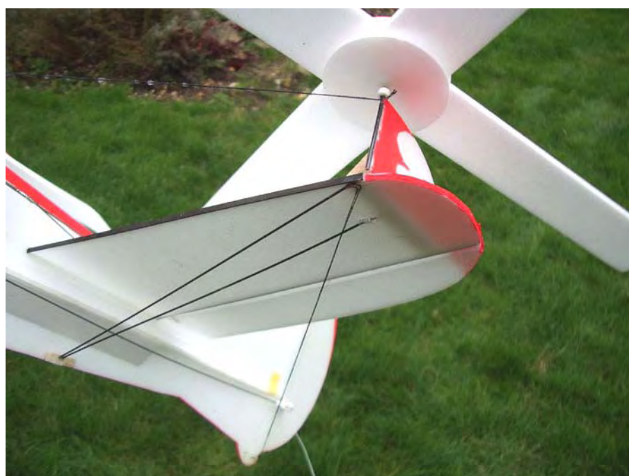
Rear wing struts and thread bracing.
