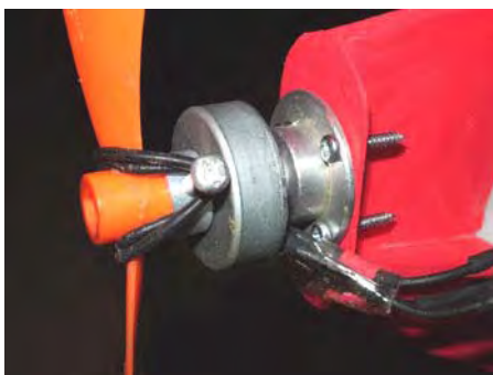
A 50 Watt CD ROM- based motor was used on the prototype
