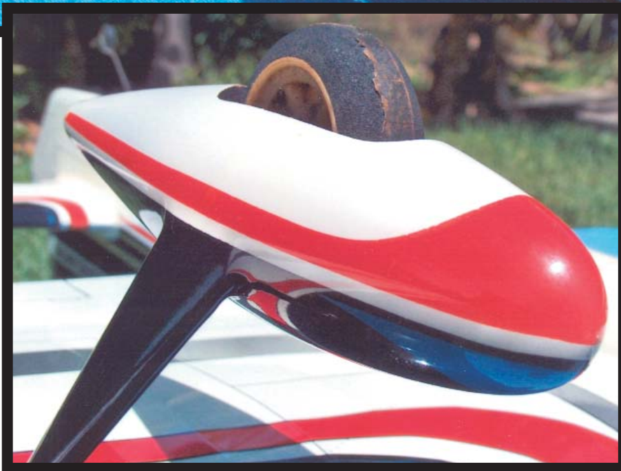
Above: In this photo of the business end of the 1982 Stiletto, you can see the cowl treatment and specifically the very cleanly-done exit hole for the muffler manifold. The very subtle intakes on the rear of the cowl were functional.
