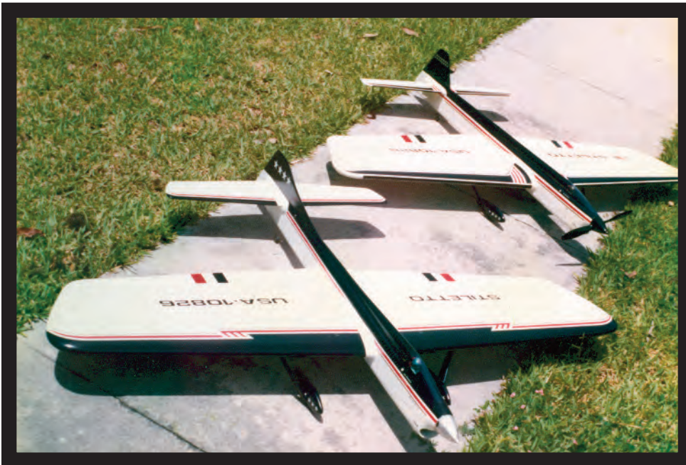
Stiletto #6 in the foreground and Stiletto # 5 in the background: The top block and vertical fin shape differences are very noticeable in this comparison shot.
