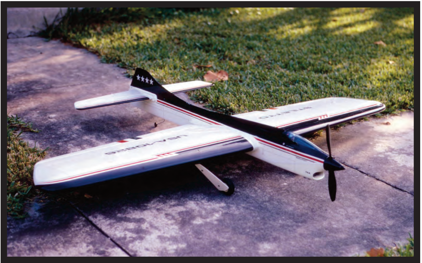
Stiletto #6 was a departure in design for Les. He incorporated a tapered top block and a new vertical fin shape. He went back to the straight top block configuration for the remainder of the models in the Stiletto series.
