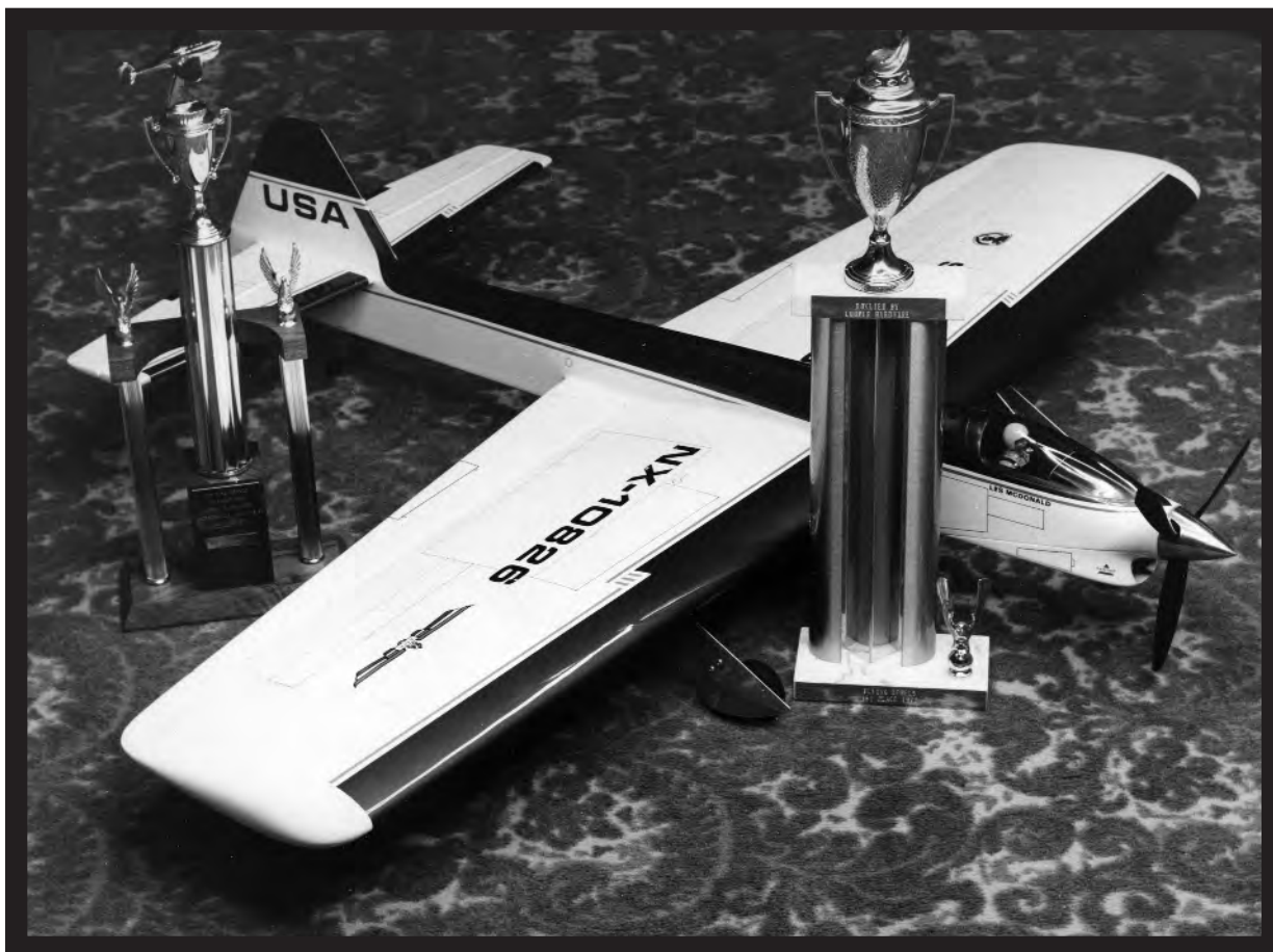
Here is the first Stiletto. It used a modified version of Jim Kostecky's Formula S wing and was powered by a Fox .35.
