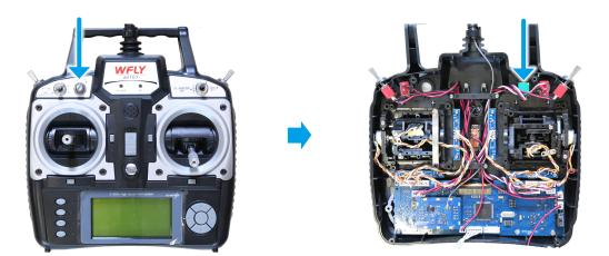
2. Pull the potentiometer down, and use the electric iron to solder down the potentiometer connection cable. Solder switcher connection cable to corresponding potentiometer cable. Do the insulate protection by heat shrink tube or insulating tape.
