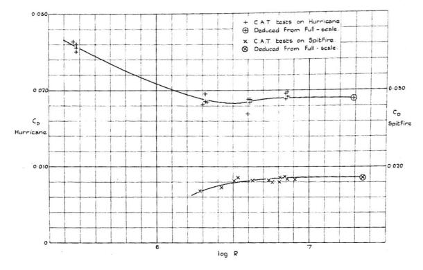
Figure 3 Drag coefficient, C<sub>D</sub>, variations with Reynolds number, R, for Spitfire & Hurricane models. Collar <sup>(26)</sup>
