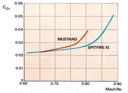
Figure 4 Variation of C<sub>D0</sub> with Mach number for the Spitfire PR XI and the P-51 Mustang, from Quill's contribution to Reference 7
