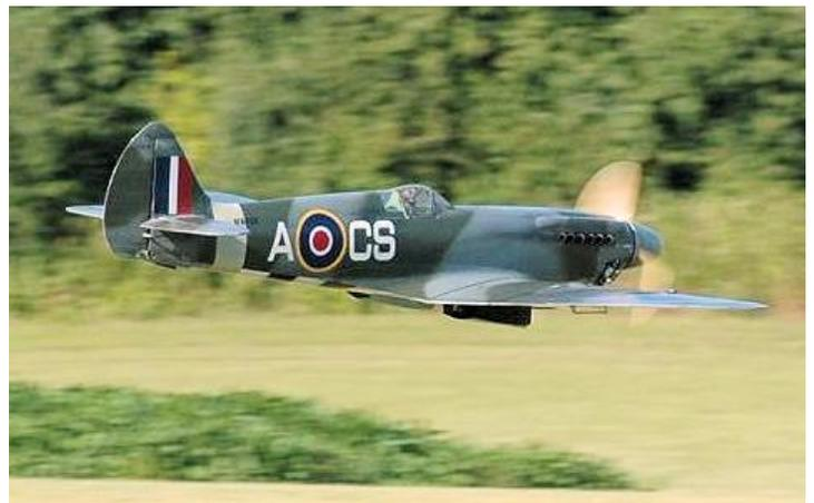
Despite its thin and pointed wingtips, Dave Szabo's Spitfire has excellent handling due, in part, to about 2 ½ degrees of washout, slightly more than the full-sized Spit. Low pass before a chandelle shown here.
