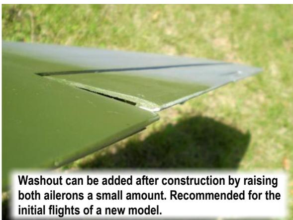
Washout can be added after construction by raising both ailerons a small amount. Recommended for the initial flights of a new model.
