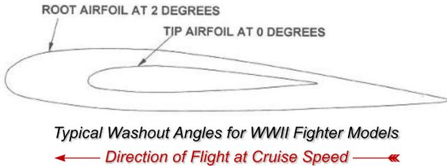
Washout is a twist in a wing that causes the wingtip to meet the airflow at a lower angle than the root in normal upright flight. Some planes don't need it; some planes can't fly without it. It's not just to prevent tip stalls!
