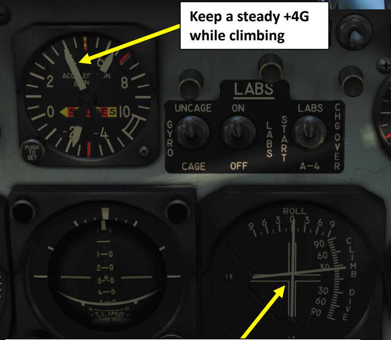
Keep yourself aligned and avoid rolling movement by checking the LABS gyro reference lines
