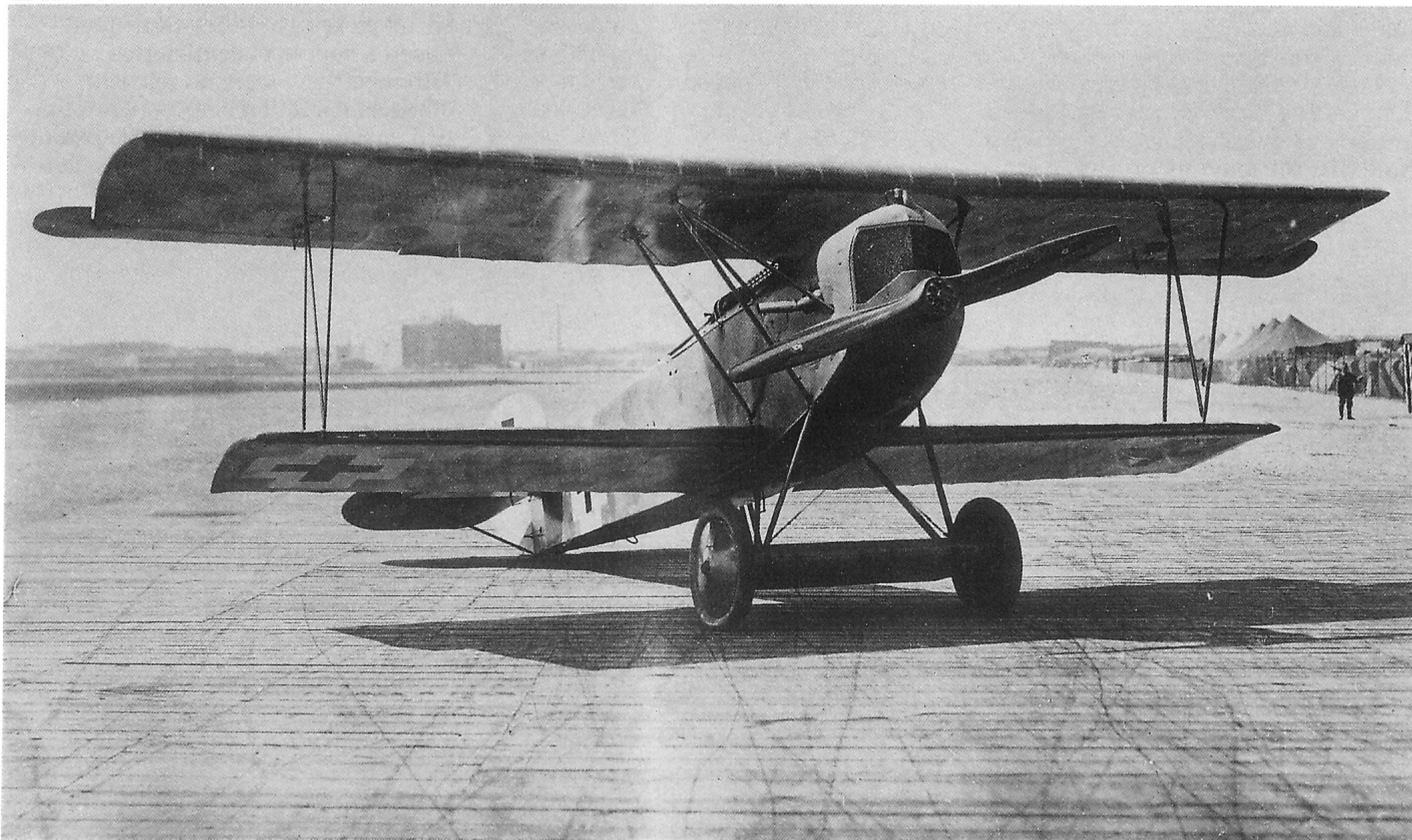
J. Overleaf, a fine shot of 527/18 reveals the hinged and split undercarriage wing, offset wheels, level exhaust tailpipe, and two spar identification windows in the underside of the upper wing - all Albatros features. The trailing edge of the panel under the engine has lost its pristine outline. (Albatros/P L Gray)
