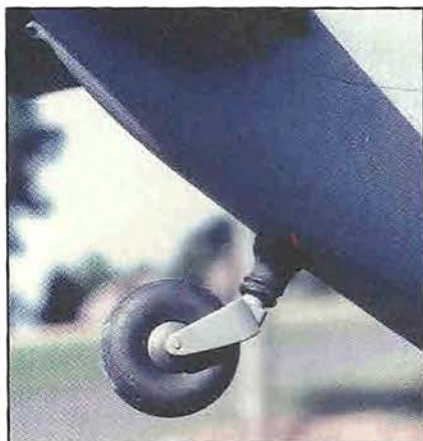
Scale Lyte-Flyte tail wheel. Boot is molded silicone glue.
