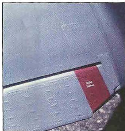
Glue-drop rib stitching on flap simulates fabric covering.
