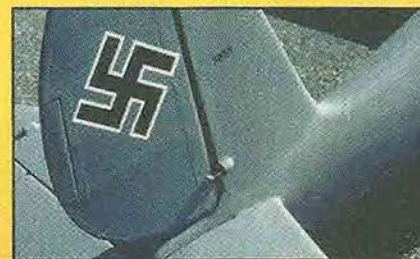
Scale rudder cables aren't real. Operational cables are inside fuselage.
