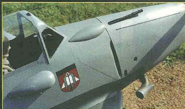
Scale surface rivets, panels, holes, hinges, etc., add realism.
