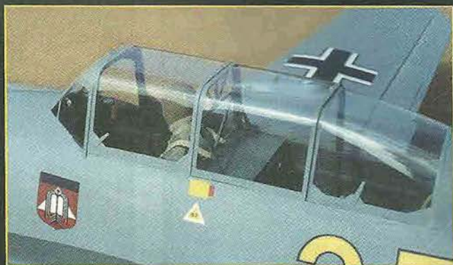
Vacuum-formed canopy available from Aerotech Models.
