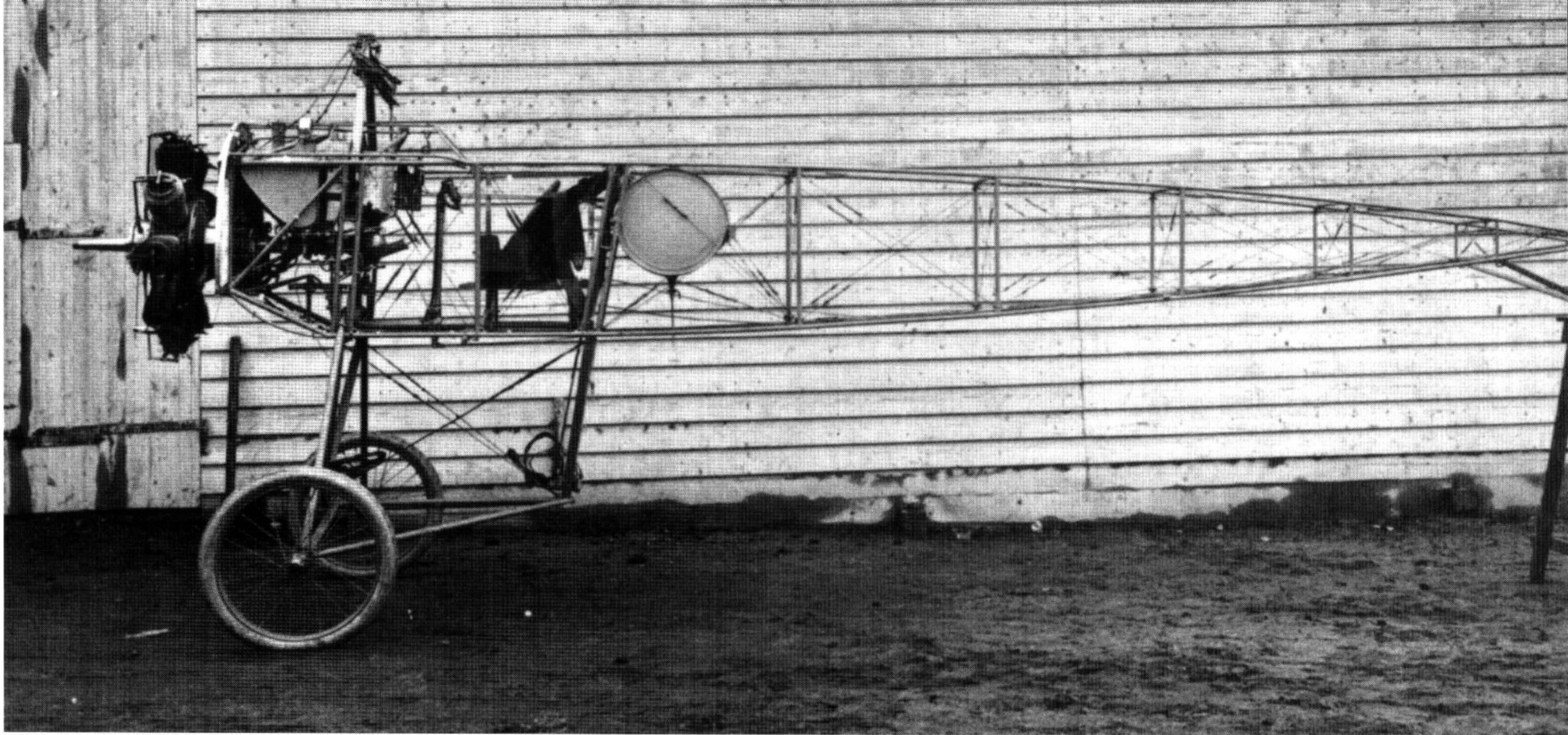
This uncovered Fokker E.III airframe reveals the placement of the pilot's seat, control stick, gas tank, engine and ammunition storage bins. (Grosz)
