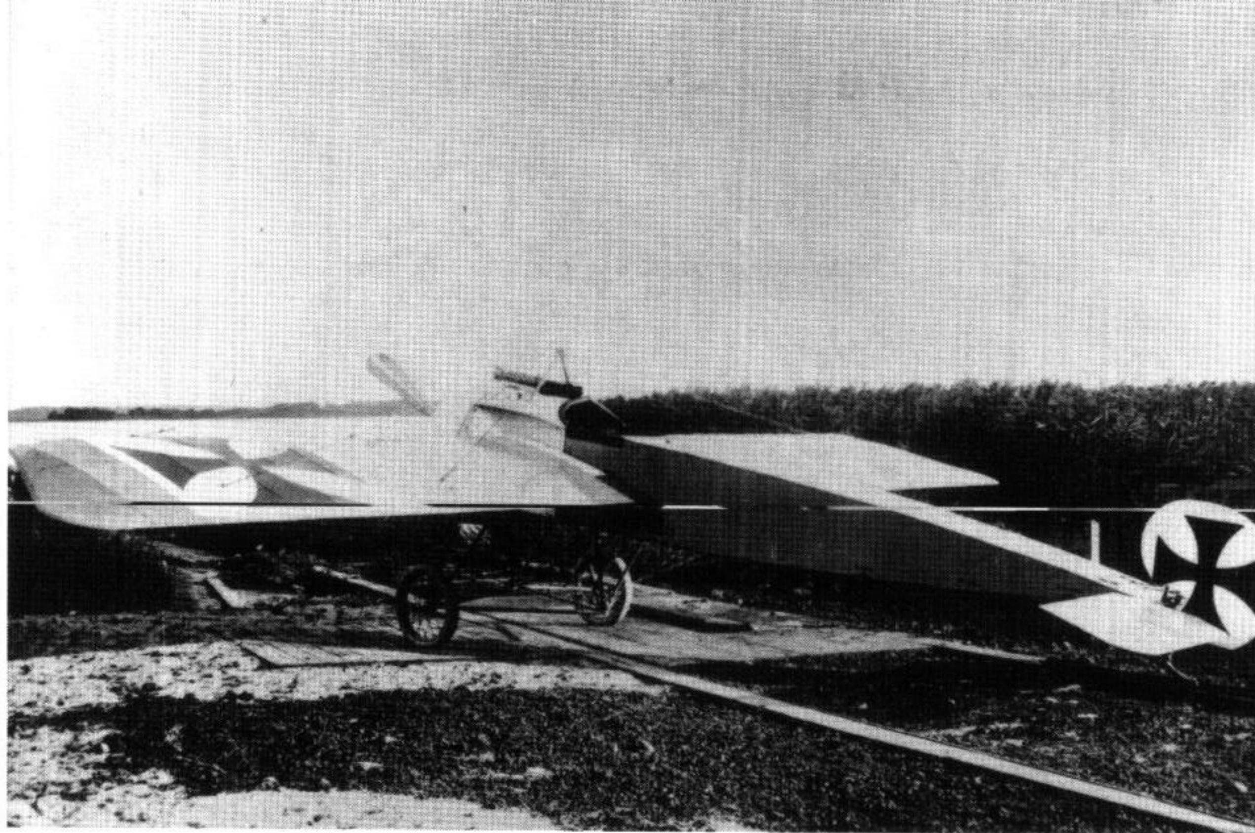
M.14 (E.II) 69/15 parked in the open near the Fokker factory. This may have been the last Fokker E.II to be produced. (R. R. Martin)
