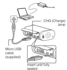
3 When charging is finished, delete the USB connection between the camera and the computer (page 53).
