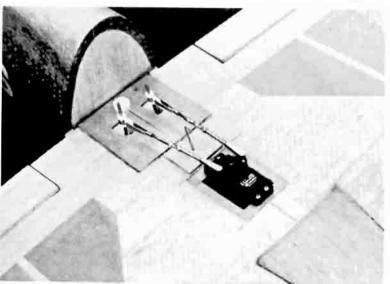
Wing centre section shown aileron servo mounted on wing top surface with clevis connections is the strip aileron control horns.
