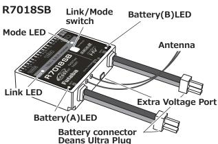
Use a Deans Ultra Plug with the R7018SB power supply battery. Batteries of this connector cannot be used.
