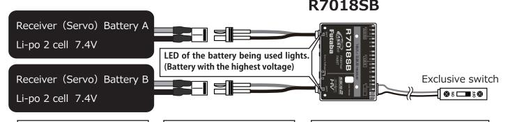
Even if the voltage of one of the batteries drops, power is supplied from the other battery. Even if the power supply wiring of one of the batteries breaks, power is supplied from the other battery.
